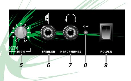
**7: HEADPHONES:** Use this jack to connect headphones to the amplifier. The internal speaker is disconnected when headphones are used.
